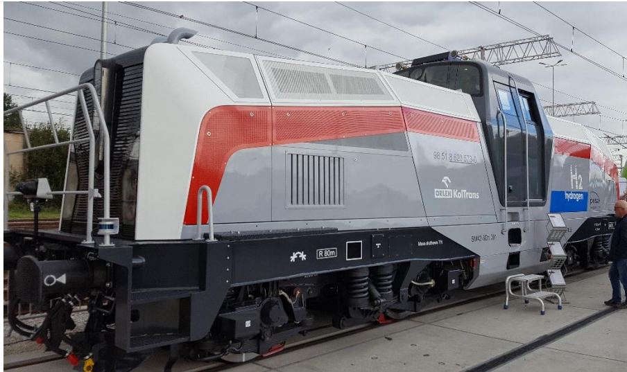
Fig. 2. The SM42 6Dn hydrogen locomotive presented at the TRAKO 2021 fair in Gdańsk (source: [22])
