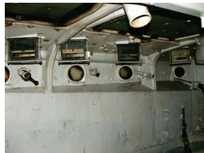
Fig. 5. View of the combat and landing compartment after removing the elements of the arming and disassembling the ball joints
