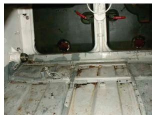
Fig. 7. View of the landing compartment after dismantling the fuel tank and depriving the tanks of the landing craft
