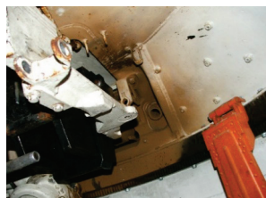
Fig. 5. View of the combat and landing compartment after removing the elements of the arming and disassembling the ball joints
