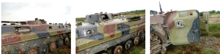
Fig. 4. View of the BWP- 1 infantry fighting vehicle with holes in the hull of the vehicle and turret and dismantled covers of the shooting holes
