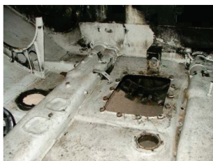
Fig. 6. View of the driving compartment after disassembly of the engine, gearbox and removal of the clamping legs
